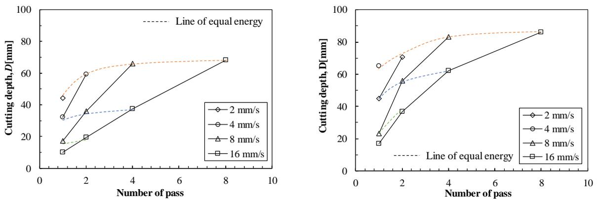
(a) Water flow rate of 30 mL/s and abrasive flow rate of 7 g/s (b) Water flow rate of 50 mL/s and abrasive flow rate of 10 g/s
