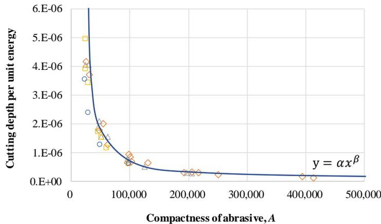
Fig. 5 Rock cutting model considering traverse rate and cutting efficiency
