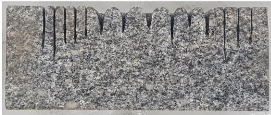
Fig. 3 Cutting result on the rock depending on the traverse rate
